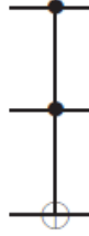
Figure 3: The Toffoli Gate (or CCNOT gate) with control in the first two qubits
